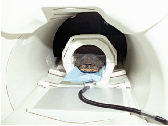
FIGURE 86-5 The closed magnetic resonance imaging (MRI) machine has a donut-shaped magnet as its largest component. It produces and sends and can receive signals. For small-bodied animals like this turtle, a smaller receiver coil mounted inside the gantry provide better images.
