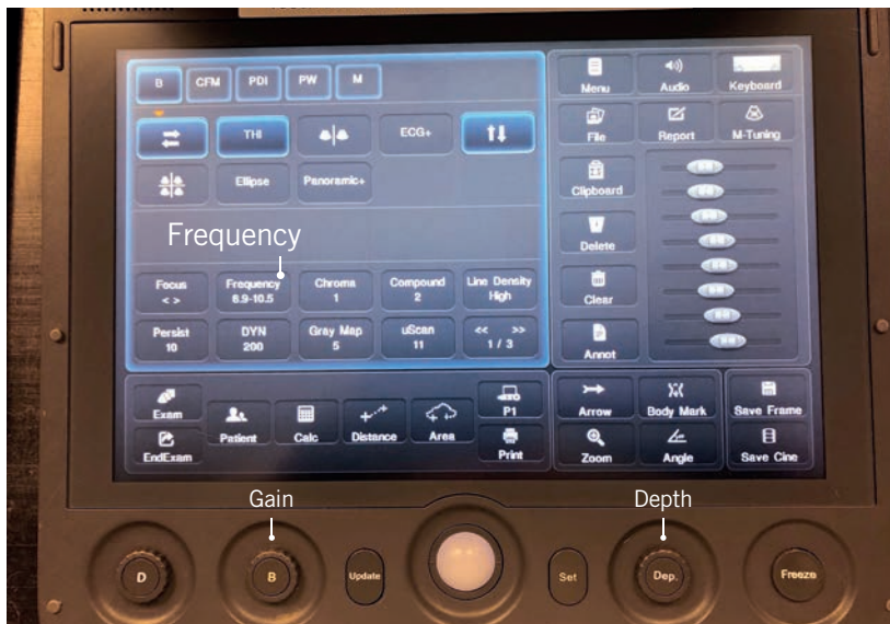
Figure 1. Typical ultrasound machine keyboard. The 3 main ultrasound machine functions used during POCUS examinations: gain, depth and frequency. The gain is used to make an image sharper and to highlight different structures and fluid. Depth is used to change how deep the ultrasound beams go and what is visible on the screen. The frequency setting of the transducer will affect image quality and depth perception.
